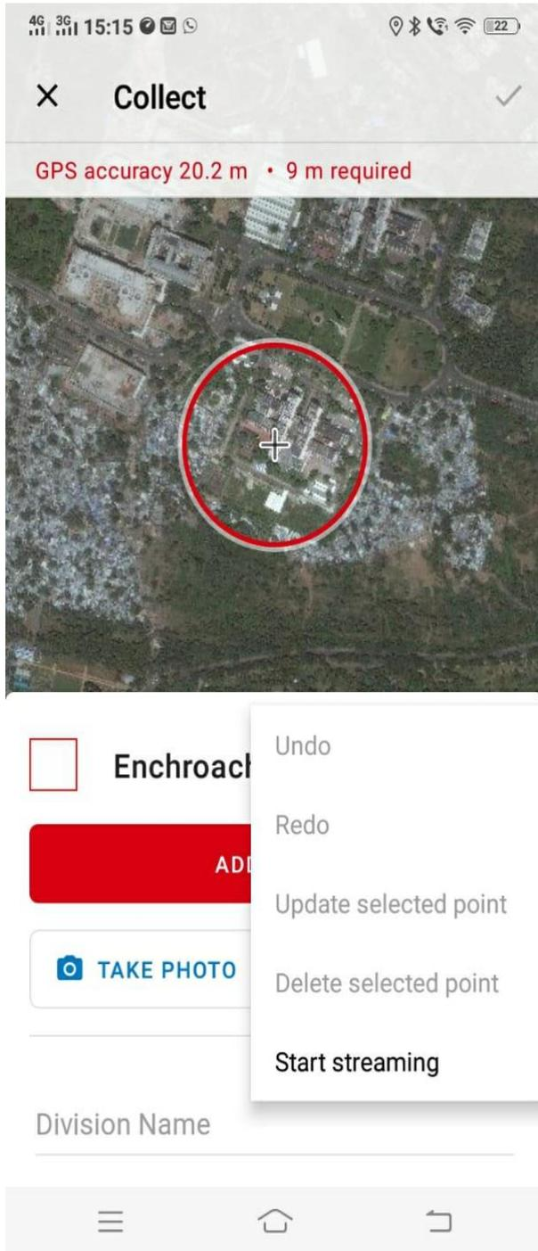
(8) Now where you walks surveyed line created automatically. To stop the survey **tap on stop streaming** here you can capture/attach the photograph of surveyed area as shown below-
