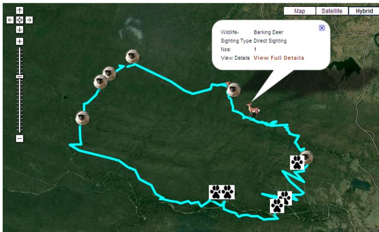
The application automatically picks up the geo-location of the sighting or evidence location with the date and time. The application also facilitates to open the digital map (in ESRI Shapefile format) as background layers. When the party finishes the patrol, the captured data is uploaded on to the server through data synchronization application.
